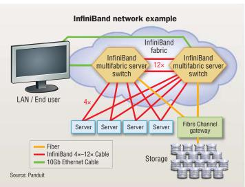
nector is based on a precision screened and balanced edge card design. InfiniBand channels are commonly deployed in point-topoint configurations to help InfiniBand networks, such as the one illustrated here, use 4X and 12X cables engineered specifically for the protocol.
