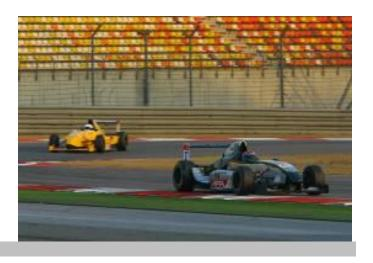
The Formula Renault 2.0 features approximately 200hp in a chassis of only 490kg, giving an extremely high power to weight ratio. Combined with effective aerodynamics, the car is similar to Formula 3.
