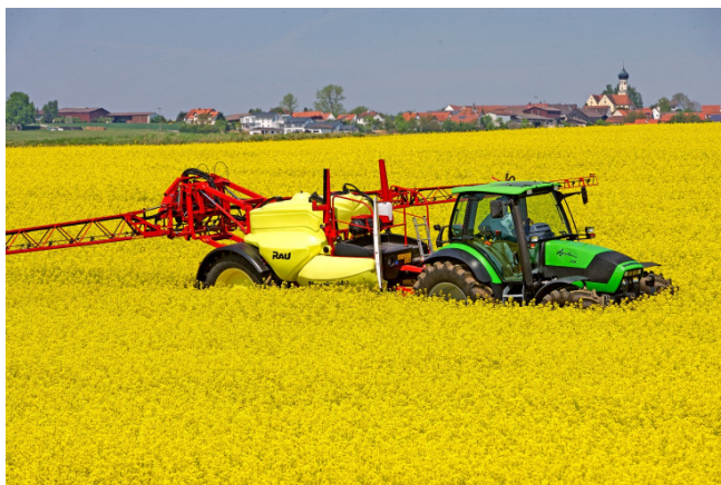
DEUTZ-Fahr Agrotron Natural Power (TCD 2012 L06-4V 133,5 kW / 2100 min -1 )
