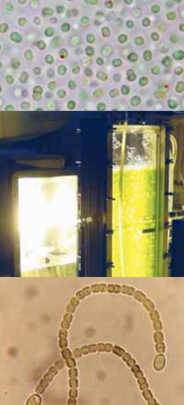
Microorganisms that can produce hydrogen from solar energy and water: Synechocystis (top) is a unicellular cyanobacterium; Nostoc (bottom) is a filamentous cyanobacterium, which also can transform atmospheric nitrogen into vital nutrients. The cyanobacteria are grown in a tailor-made bioreactor (middle), where light intensity, temperature and nutrients are carefully monitored. In the future, vast bioreactors filled with cyanobacteria could become a source of hydrogen produced biologically from sunlight and water.
