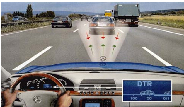
Driver's view to the Distronic display and Distronic control unit and radar sensor
