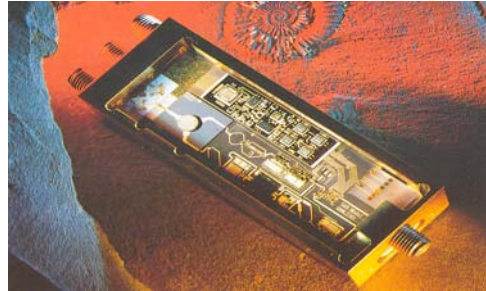
AMSAR demonstrator and X-band TRM
