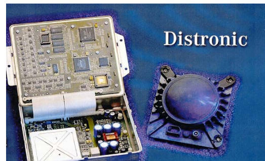
Driver's view to the Distronic display and Distronic control unit and radar sensor
