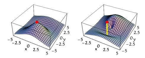
He  $1 \text{ s2p}_y$  Fermi heap (left) and Fermi hole (right). The post marks the position of one electron, at  $y = -2 a_0$  in the xy plane. The height of the surface is the probability density of the other electron. The Fermi heap shows the clumping of the two electrons, while the Fermi hole shows that the two electrons are never found in the same place.
