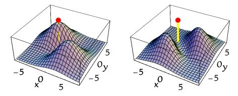
C 2  $p_x$  2  $p_y$  Fermi heap (left) and Fermi hole (right). The post marks the position of one electron, at  $(x, y) = (-2\sqrt{2}, 2\sqrt{2}) a_0$  in the xy plane. The height of the surface is the probability density of the other electron. The Fermi heap shows the clumping of the two electrons, while the Fermi hole shows that the two electrons are never found in the same place.
