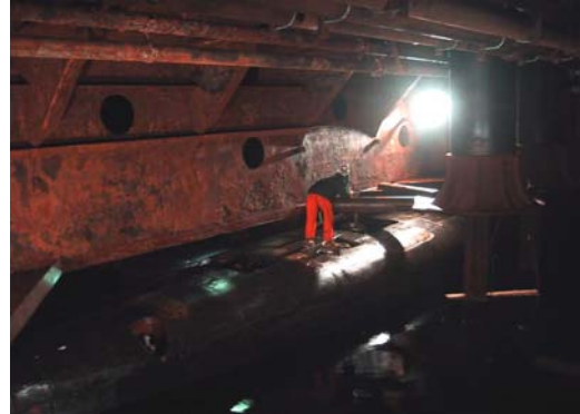
Checking the Sail for Radioactivity The sail (conning tower) of the Kursk protruding up into the cavity formed in the underside of the Giant 4
