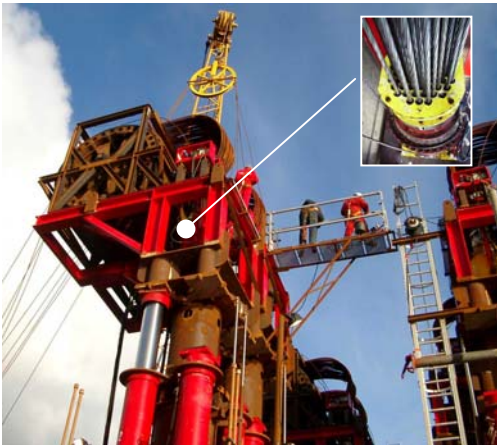
The strand jack (inset) mounted within the cable reel platform with the swell compensator rams underneath
