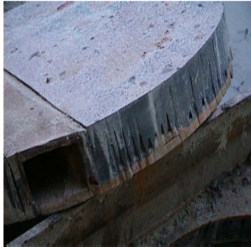
The External Acoustic Layer, showing Noise/Sonar Attenuation Voids revealed by the cutting of the lifting sockets
