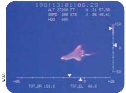
Space Shuttle Discovery during STS-121 entry obtained by Navy Cast Glance infrared sensor.
