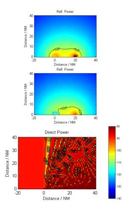
All results are calculated for the source pointing towards the target. The top result, 'reflected power', is for the source  $\rightarrow$  target  $\rightarrow$  receiver path, whereas the bottom result, 'direct power', is the direct source to receiver path and is independent of target height.
