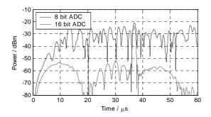
This shows clear target detection for the higher dynamic range receiver with identical noise levels between simulations.
