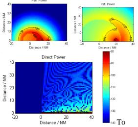
provide an increase in target detection range, a higher gain receive antenna could be used. The result for a 20dBi antenna is shown below.
