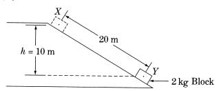
A 2 kg block, starting from rest, slides 20 m down a frictionless inclined plane from X to Y, dropping a vertical distance of 10 m as shown above.
