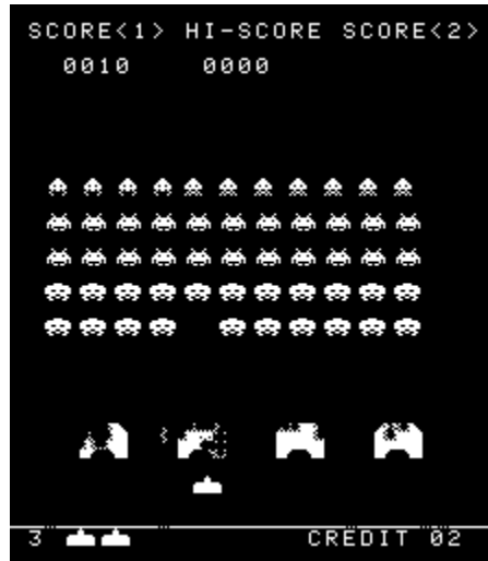
Fig. 8b. A snapshot of Space Invaders ' video RAM during play after 270 degree rotation. Note that black pixels are 'off' (0) bits and white pixels are 'on' (1) bits.
