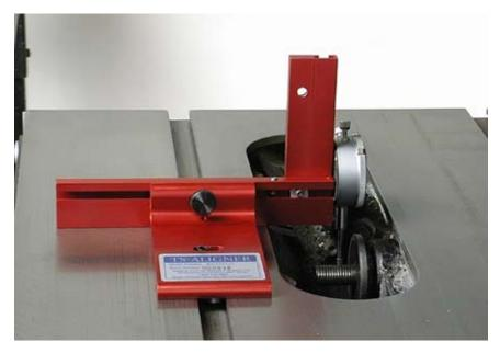
with the arbor and the dial indicator reads about mid scale. Establish a reference point by rotating the scale so that the large hand points to zero.
