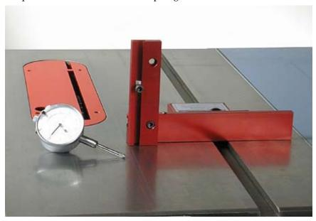
The dial indicator then connects to the Upright Bar using the supplied 1/4-20 socket head screw and nut as shown in the following photo.
