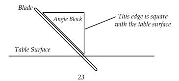
With TS-Aligner on the table, push the Cross Bar so that both stylus points are against the edge of the angle block. When the dial indicator reads exactly the same as your **One Inch Point**, then the blade is tilted to the correct angle.
