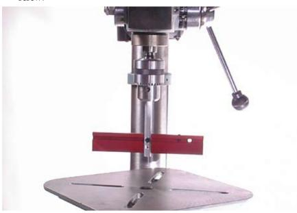
Now attach the Upright Bar to the Cross Bar so that it extends upwards as shown in the next photo.
