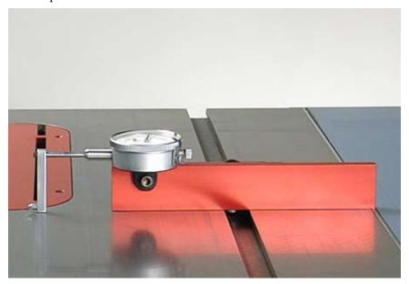
The dial indicator should be tilted so that it rests against the setscrew on the top of the cross bar. Each dial indicator is slightly different and sometimes the bottom of the stylus offset will drag on your table surface. If this is the case, just file the bottom of the stylus offset bar until it no longer drags. DO NOT ADJUST THE SET SCREW ON THE CROSS B AR UNDERNEATH THE DIAL INDICATOR. This screw controls calibration for angle measurement.
