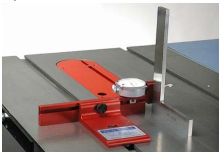
Finally, place the blade of the square against the upper stylus point (the one attached to the plunger on the dial indicator) and push it in
