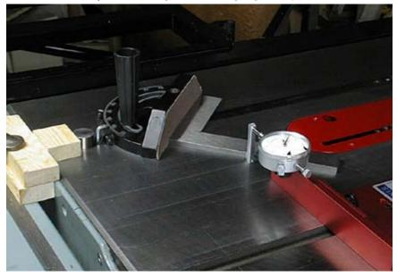
The above picture shows the setup with the spacer block in place. Make sure TS-Aligner Jr. doesn't move while you make this adjustment. If you find this adjustment tricky you are not alone. Even with practice it's fairly cumbersome. For greater accuracy, you will need to use the
