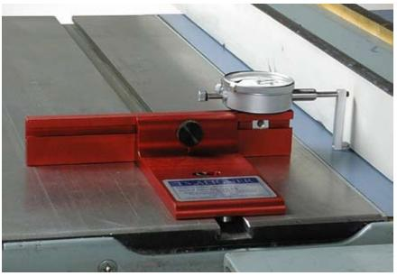
If the front end of the fence reads differently from the rear end, you may need to adjust it so that the two ends read the same. If your blade
