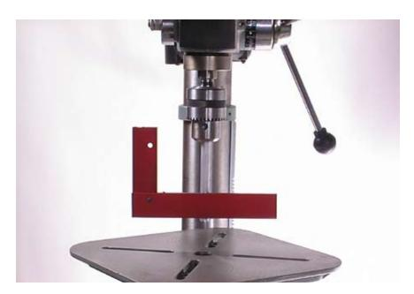
Finally, attach a round or domed stylus tip to the Dial Indicator and mount the Dial Indicator to the Upright Bar so that it points downwards. The photo below shows how it should look.
