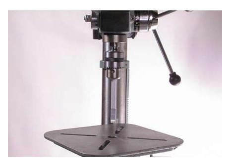
Next, mount the Cross Bar onto the Spindle Rod using the thumb-screw.
