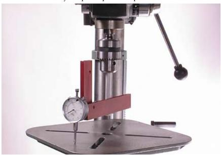
The next test you will want to perform can tell you how true your drill chuck and spindle rotate. This is refered to as measuring the spindle runout. It will also give you an idea of the condition of the spindle
