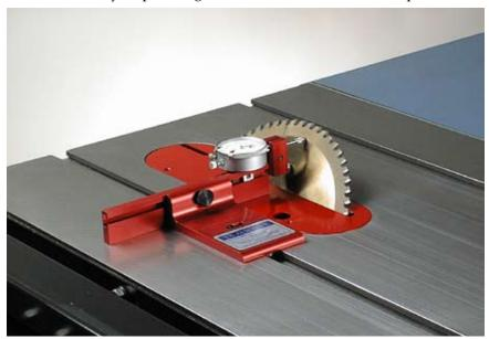
If the reading on the dial indicator doesn't match the value in the table, then you will need to adjust the blade tilt. With the Cross Bar knob loosened, push in so that both stylus points remain against the blade. Then adjust the blade tilt until the reading on the dial indicator matches the value in the table. Be sure to keep the Cross Bar flat on the table surface.
