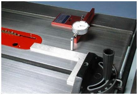
a change in reading and adjust the angle of the miter gauge to obtain the minimum amount of change. Always move the miter gauge and leave TS-Aligner stationary. If you move TS-Aligner and leave the miter gauge stationary, you will be aligning the miter gauge so that it is square with the slot that TS-Aligner is in.
