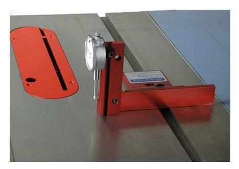
The dial indicator can then be adjusted up and down along the slot in the Upright Bar. Remove the throat plate and blade from your saw.
