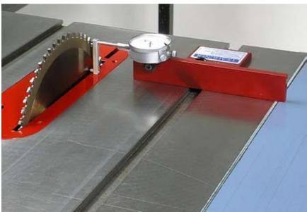
4. As little as 0.005" change in reading can adversely affect the quality of your cuts. Some saws require that you move the table surface. Others have you shift the trunnions. Refer to your saw's manual to determine how the adjustment is made (it is sometimes referred to as adjusting the "heel" of the blade). You can leave TS-Aligner Jr. in contact with the blade while you make
