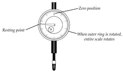
this small knob, you will be able to rotate the scale freely so that the zero point can be placed at any position that the large hand sweeps.
