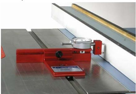
For this test you will need to install the Angle Attachment Gage and have it calibrated at the **One Inch Point.**
