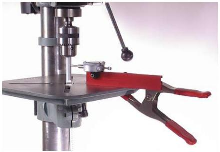
Establish a reference point with the stylus of the Dial Indicator in contact with the Spindle Rod. Now manually rotate the spindle and observe the reading on the dial indicator. A reasonable quality drill press with a good chuck will have no more than 0.002" of runout. If the reading jumps as you place side pressure on the chuck, you have some play in the bearings.
