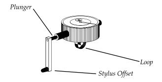
To assemble, attach the stylus offset to the plunger on the dial indicator by first removing the screw that is already on the end of the plunger. Place this screw thorough the hole in the stylus offset and screw it back into the plunger.
