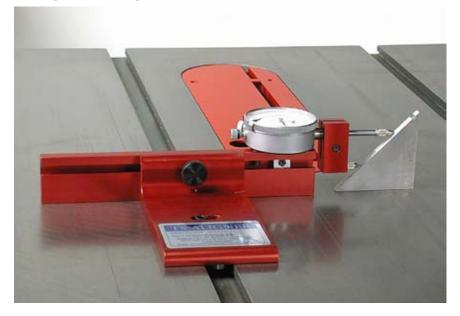
First, check the <u>One Inch Point</u> by using a square as described in the previous section. Make sure that the dial indicator is resting firmly on the Tilt Adjustment Set Screw (the dial indicator is tilted all the way back). Adjust the position of the Angle Attachment Gage on the dial indicator stem so that both hands point to zero when both stylus points are against the edge of the square.
