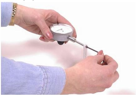
DO NOT OVERTIGHTEN THIS SCREW! The plunger on the dial indicator is not designed to take radial forces and THE INTERNAL MECHANISM CAN BE EASILY DAMAGED. Tighten the screw only tight enough to keep the stylus offset bar in place. Due to differences between each dial indicator, this screw may not go in far enough to clamp down on stylus offset. If this happens, just file or grind down the screw until it fits. UNDER NO CIRCUMSTANCES SHOULD YOU EVER TRY TO FORCE THE SCREW.
