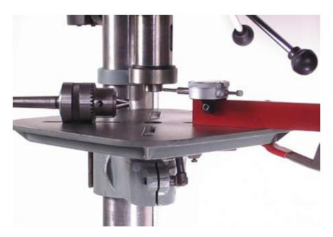
Actual spindle runout on a reasonable drill press will be less than 0.001". See your owner's manual for details on how to remove the chuck.
