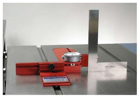
Next, place the blade of the square against the side of the Angle Attachment Gage. Rotate the Angle Attachment Gage on the dial indicator stem until it is square with the table surface as shown in the following photo.
