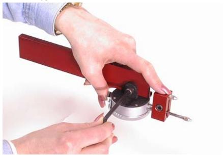
This ensures that the dial indicator is firmly resting against the calibration set screw.
