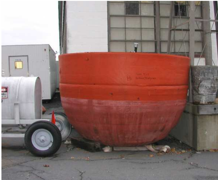
Figure 4: The reusable foam section of the buoy located at the NRL site near Chesapeake Beach, MD.
