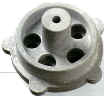
This valve cap used in aircraft equipment includes multiple wall thicknesses and cast-in holes. Alloy: 356 aluminum, 0.515 lbs., shown 1/2 actual size.
