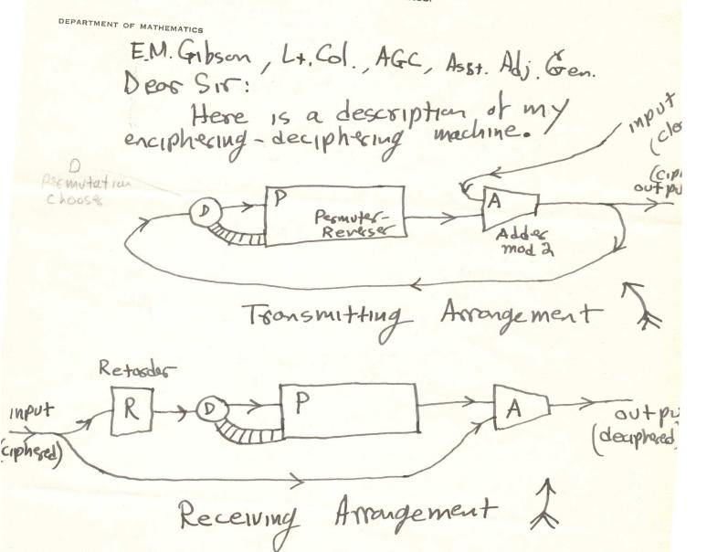
In the receiving arrangement the same components one used except for the addition of the retorder, which is a one-onit delay. The messages are to be sequences of binoxy digits (numbers mod 2). The machines work on a cycling basis, performing certain operations
