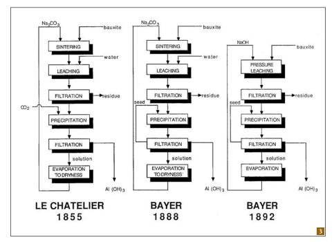
Fig. 3. The shift from the thermal route (Le Chatelier process) to the hydrometallurgical route (Bayer process) for the production of alumina.
