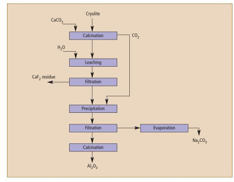
Fig. 13. Thomsen's process for the recovery of  $Al_2O_3$  and  $Na_2CO_3$  from cryolite.
