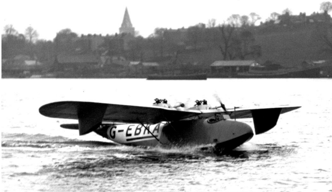
4. Short Bros. photo.H 75 (c). The Cockle motoring along on the Medway with John Lankester Parker in charge, possibly on its first outing on 18 September 1924. JLP tried for thirty-three minutes to take-off without success.
