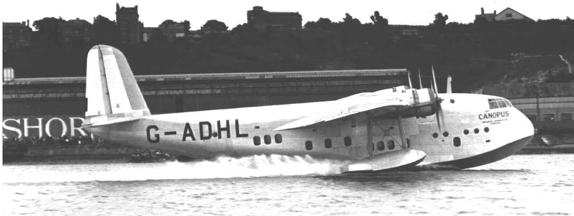
19. Short Bros. Photo H.907 (g). 'HL CANOPUS gathering speed for take off on 4 July 1936 before an assembled multitude of spectators. Note the original sprung float arrangement, the un-painted mahogany trim tab, the lack of the upper servo tab on the rudder and the original position for the owner and port of registration lettering.
