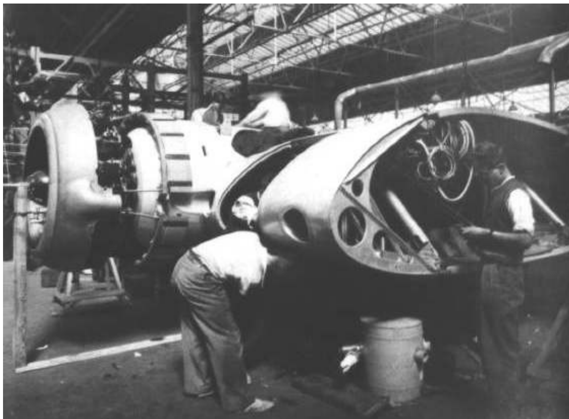
30. Short Bros. photo H 877 showing the starboard inner engine of 'HL CANOPUS' fixed in position on the nacelle, complete with collector ring and gills but without cowling or exhaust pipe.
