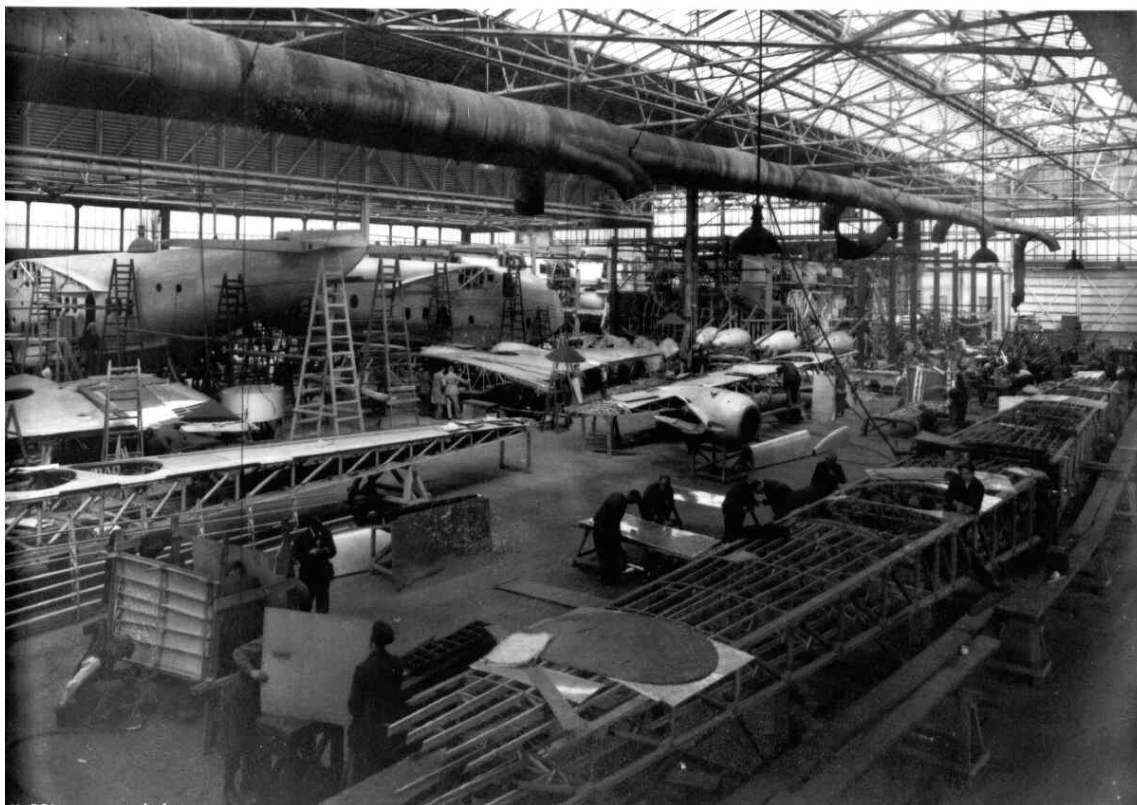
13. Short Bros. photo H 861. The completed hull of G-ADHL is in the left background, with its two half mainplanes on either side of the tail, sheeted and awaiting the installation of engines. The newly withdrawn hull of G-ADHM is in the centre background. The two half mainplanes in the centre of the photo, showing the spar truss, are for 'HM'. The mainplane spar boxes in the right foreground, ready for sheeting, are for the first Mark II 'boat, G-ADUT.
