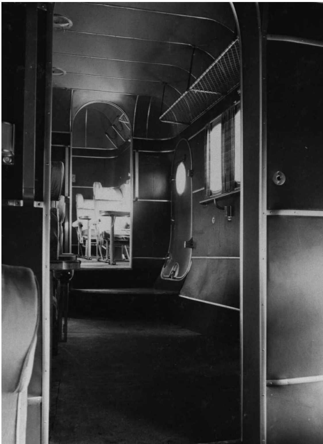
18. Short Bros. photo 8S126-3 An interior photo taken from the Centre Cabin, looking aft into the Promenade Cabin, showing the Promenade space. A combined wall and bunk light with Steward's call button is to the left of the opening. An escutcheon for the end of a bunk is to the right of the opening. The passenger entry hatch is in the centre of the photo. The Aft Cabin is in the background.
