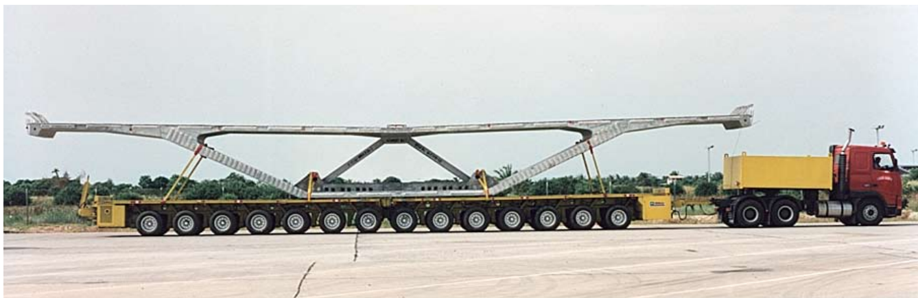
Fig. 16. D6 segment ready for transportation.
