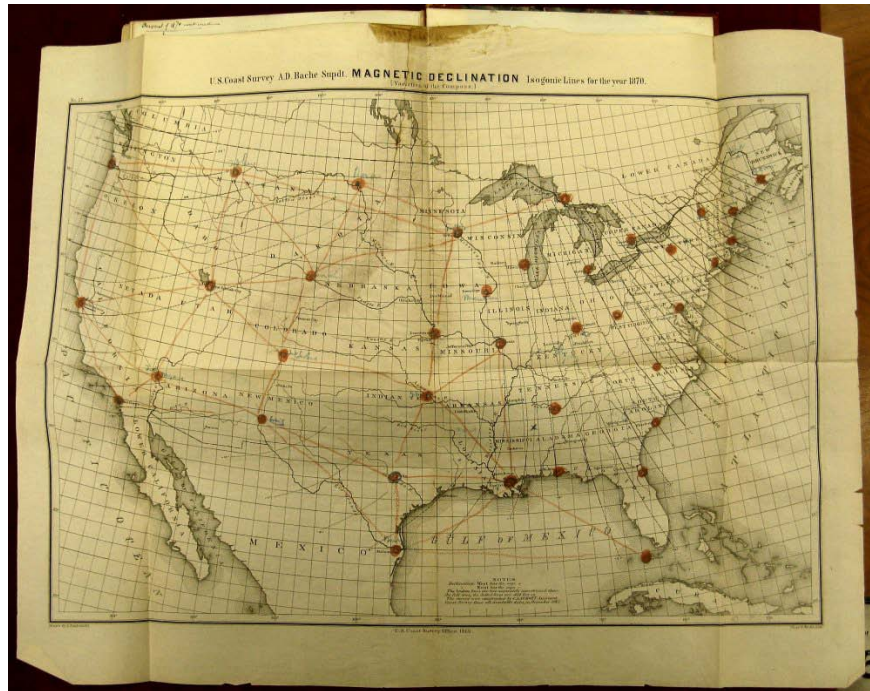
Coast Survey 1866 Sketch of Magnetic Declination for the year 1870, overdrawn by Charles A. Schott with a hypothetical network of magnetic observatories (1870-71) 14
