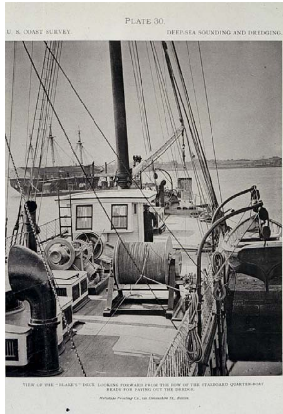
Plate 30: Steam Winch and Steel Wire on board the Survey ship “ Blake ” from “Deep Sea Sounding and Dredging” by Charles D. Sigsbee (1880).
