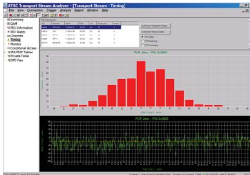
Figure 5.4 The DTS-330 Timing Display tracks PCR jitter and spacing over time
