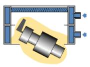
After cooling, the vacuum is released and free-flowing sand drops away leaving a clean casting, with no sand lumps. The sand is cooled for re-use.
