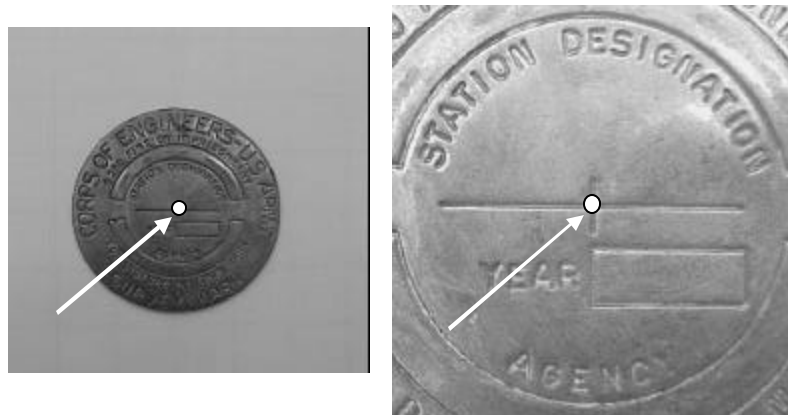
Figure 4-3. Comparison of optical plummet centering devices. The left-hand image shows the field-of-view and centering circle for a standard optical plummet fixed-mounted in a tribrach. The right hand image shows the greater magnification and centering ability provided by a nadir plummet instrument. Both images show the same brass disk at an instrument height of approximately 1.5 meters
