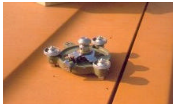
Wild tribrach with forced centering device
