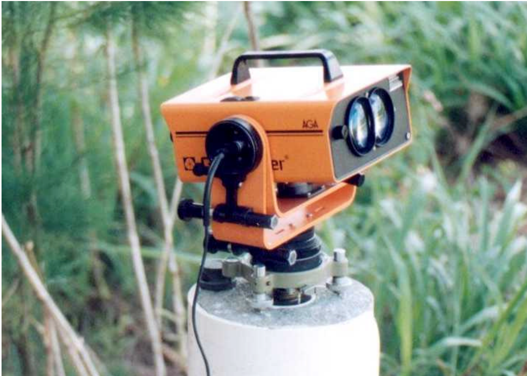
Figure 5-1. AGA Geodimeter Model 220 electro-optical distance meter mounted in Wild tribrach force-centered into rigid concrete instrument pedestal.
