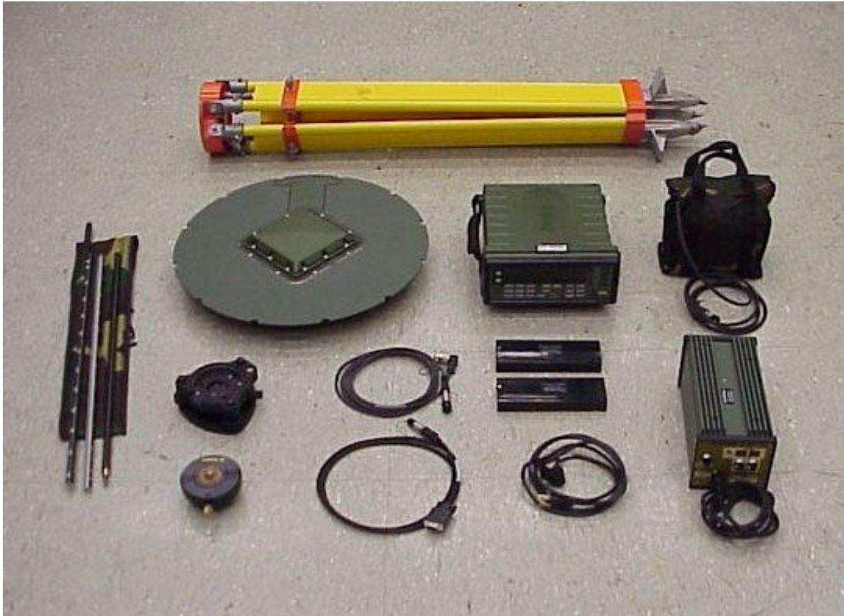
Figure 3-5. Standard GPS equipment for precise surveying. From left to right; graduated rods for antenna height measurement, GPS antenna with ground plane, tribrach, antenna/tribrach adapter, antenna cable, data download cable, surveyors tripod, GPS receiver, camcorder batteries, power cord for support module, 12V battery with attached cable, support module for data downloading.
