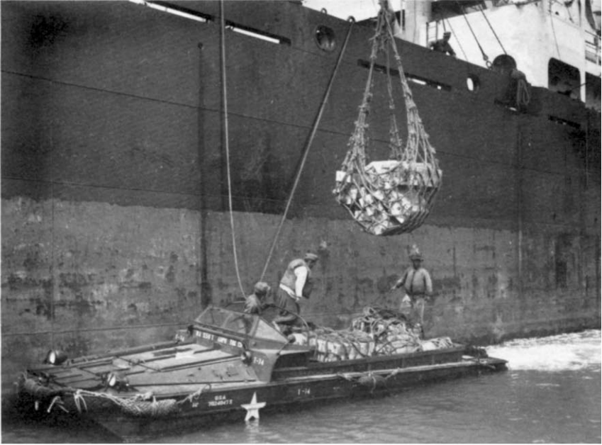
Cargo is loaded from the SS Carleton Victory to a DUKW in Inchon Harbor.
