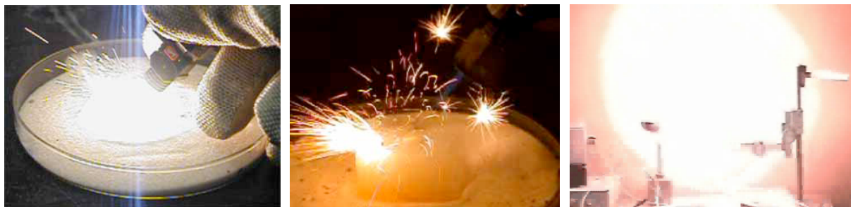
Figure 5. Still images from the thermal ignition of energetic nanocomposites comprised of sol-gel prepared \text{Fe}_2\text{O}_3 - 2\mu\text{m} Al (left), \text{Fe}_2\text{O}_3 - \text{SiO}_{3/2} -R- 2\mu\text{m} Al (middle), and \text{Fe}_2\text{O}_3 - \text{SiO}_{3/2} -R-40nm Al (right).
