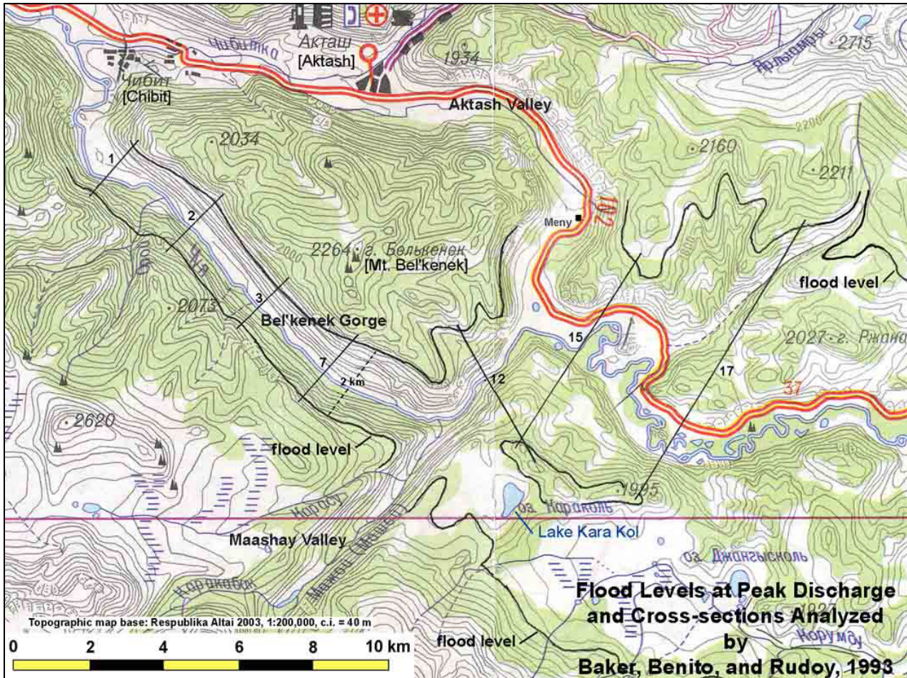
Figure 15—Bel'kenek dam area, showing the elevations of floodwaters and cross sections used by Baker and others, 1993, in their flood discharge modeling.
