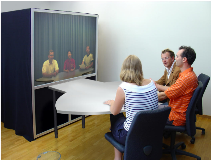
Fig. 7. The real table is extended by a virtual one, using a holographic projection screen
