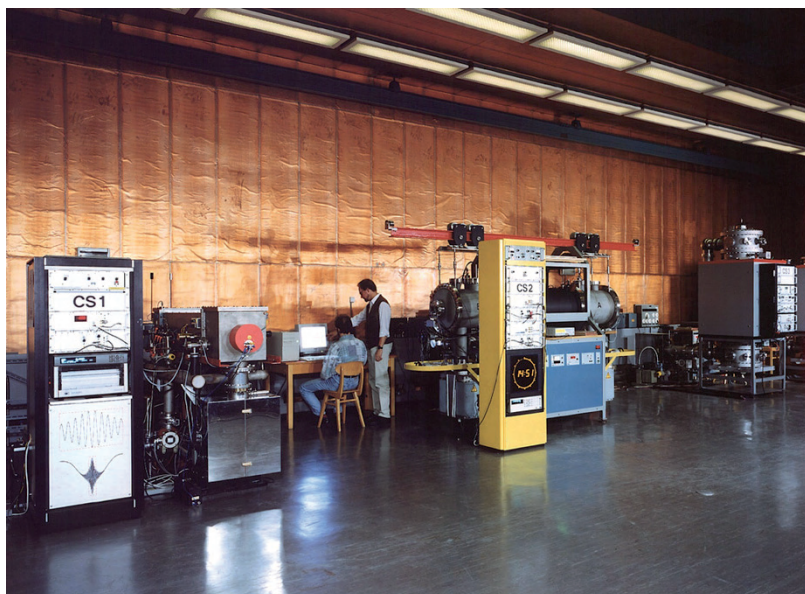
Figure 3: View of PTB's primary clocks CS1 and CS2.
