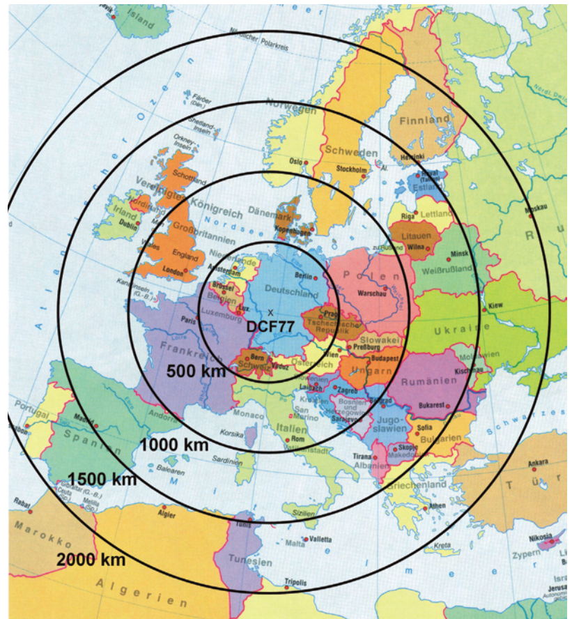
Figure 16: Schematic view of the reach of the DCF77 transmission.
