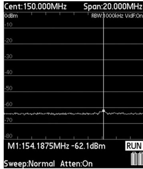
Fig. 5. Frequency resonance interaction, the far field spectral line is depressed
