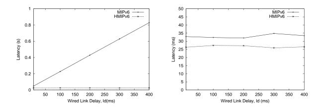
Figure 7. Impact of wired link delay on handoff latency
