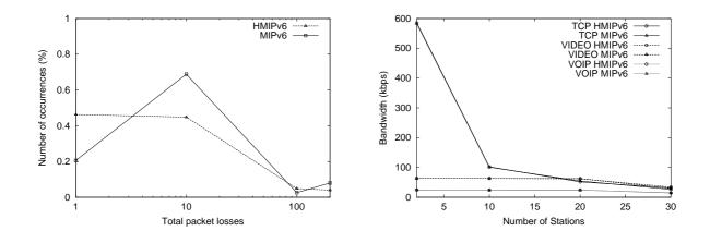
Figure 9. Histogram of the total packet losses considering random movement
