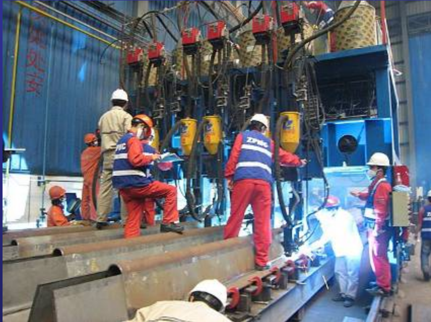
Submerged Arc Welding Gantry
