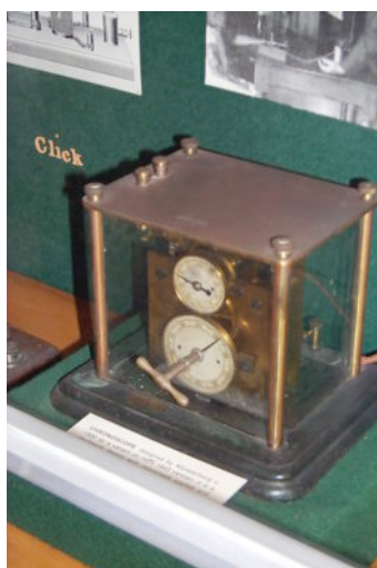
Figure 24: Münsterberg chronoscope with reset to 0, bearing no signature or serial number University of Sydney
