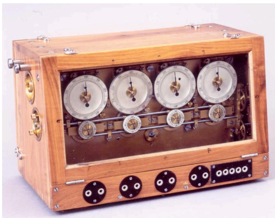
Figure 22: Chronoscope, “model 257D,” with four dials made by Favarger & Cie La Chaux-de-Fonds, MIH, Inventory No. V-226
