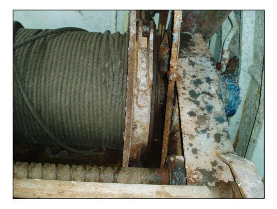
View of the starboard winch showing that the warping head is declutched.
