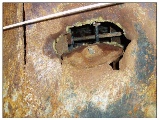
View of the breach at the port echo sounder seen from outside the vessel. The flap-like plate has pivoted into the engine room. The vertical crack in way of frame 18 can also be seen.
