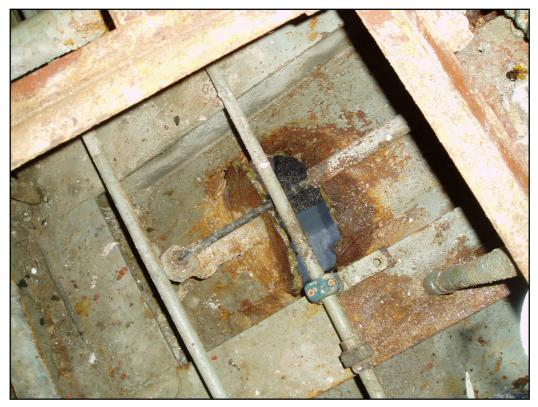
View of the breach at the port echo sounder seen from inside the vessel. On the left of the photograph the broken cable conduit coupling can be seen. The part of the conduit rising towards the upper part of the engine room is visible on the right of the photograph.
