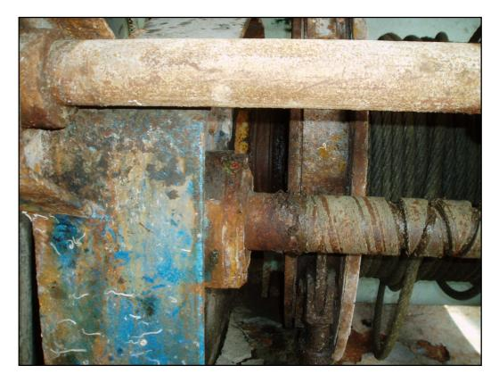
Detail of the port winch clutch jaw.
