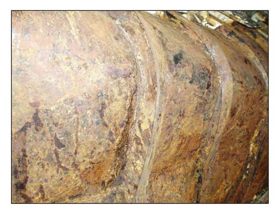
Photograph showing the deformation of the side shell and frames of the starboard side of the fish hold.
