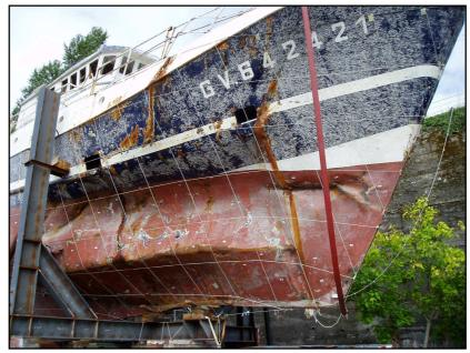
View of the deformation of the starboard side. The photograph shows the deformation in way of the fish hold and the double bottom below it. The bowing of the keel can also been seen.
