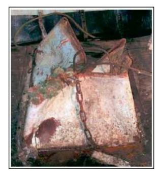
Deformation of the starboard fish hold hatchway
