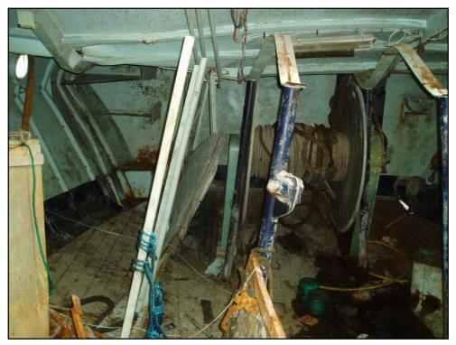
View of the deformation of the main deck. The photograph was taken from the after end of the work room.
