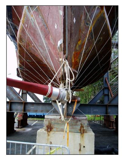
Photograph looking aft showing the symmetry of the deformations.
