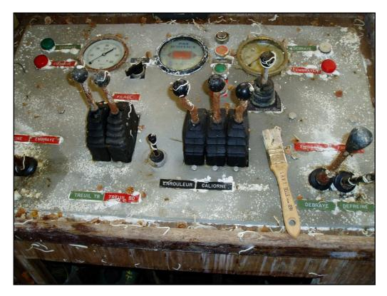
View of the winch control console on the after starboard side of the wheelhouse. The port winch brake lever is located on the far right of the photograph.
