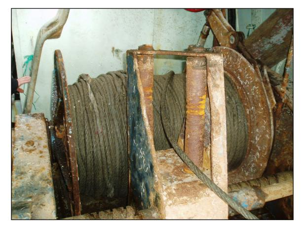
View of the starboard winch cable guide.
