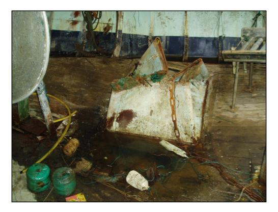
Deformation of the fish loading hatch on the the starboard side of the forward part of the work room.
