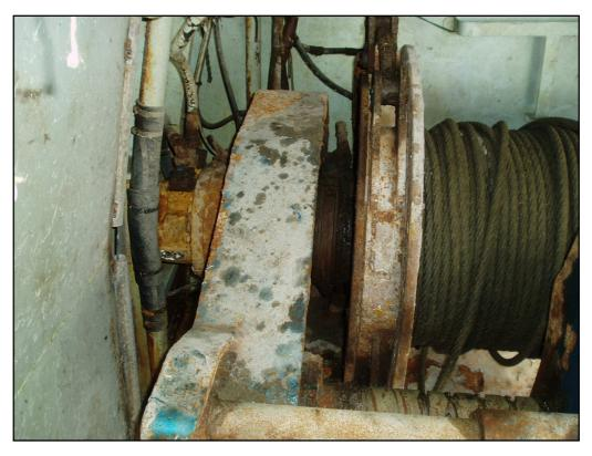
View of the port warping winch showing that the warping head is declutched.
