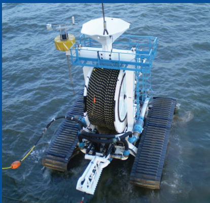
The LBT1 remotely operated cable burial machine during operations on the Lynn and Inner Dowsing Offshore Wind Farms
