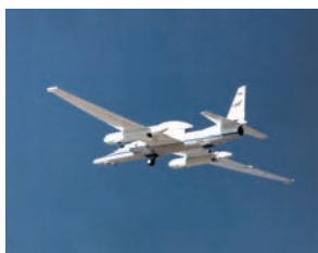
The NASA ER-2 research aircraft can carry a full range of instruments to altitudes of 70,000 feet.
