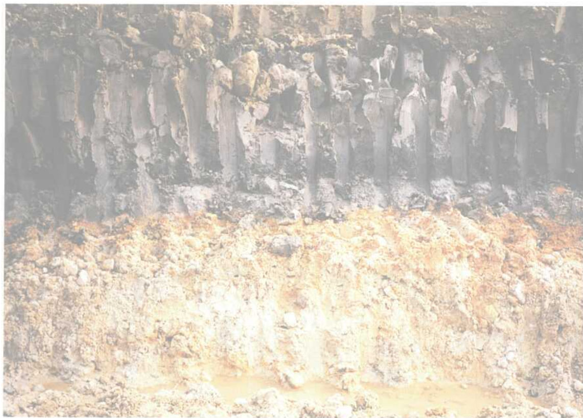
Plate 39 - Black Organic Mud, Upper Unit of Late Pleistocene Alluvial Terrace Deposits Overlying Yellowish Brown Silty Sand with Subrounded Cobbles, Lower Unit, Luen Wo Hui (3263 3972), Fanling
