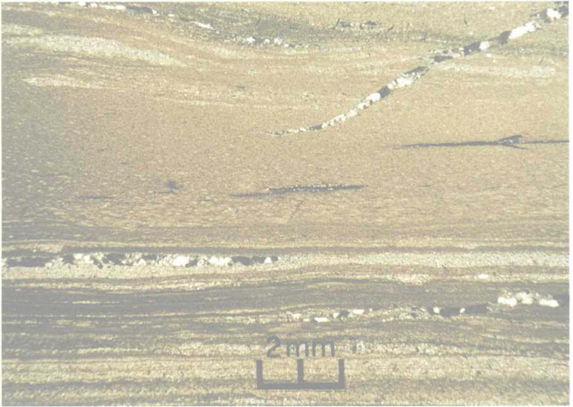
Plate 33 - Thin Section of Aegirine-bearing Laminated Siltstone (HK7314, 6190 4482), within the Ping Chau Formation, Nam Tong on Ping Chau; XPL
