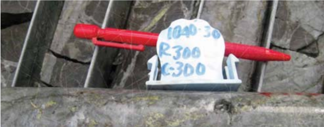
Wafi-Golpu WR333; 1 040.3 metres. Mineralised and altered diorite porphyry showing abundant chalcopyrite. Assays for this interval (1 040 to 1 041m) returned 1.4 g/t Au, 2.5% Cu.
