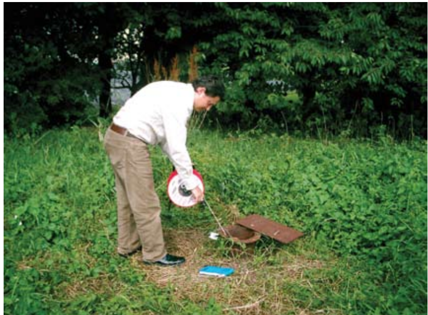
Manually checking water level in a well. Photo courtesy Peter McConvey, GSNI
