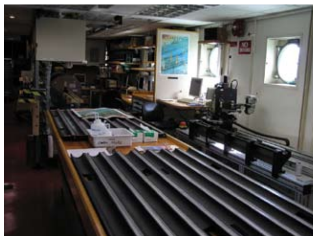
Racking for drill core
