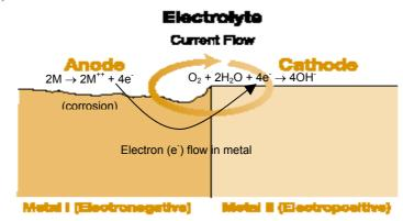
Figure 7.1. Corrosion cell / Bimetallic corrosion
