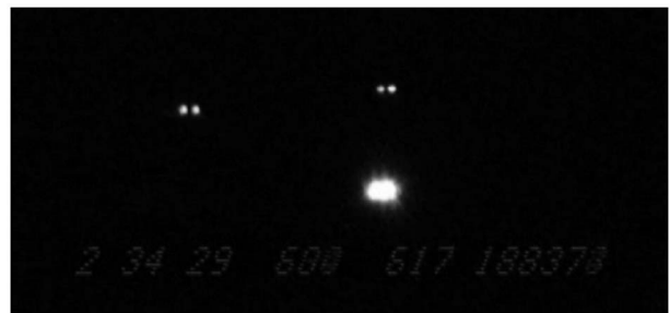
Fig. 4. Portion of video frame taken at 2:34:29 UTC 29 May 2008 (9:34:29 p.m. 28 May 2008 CDT) during period of exceptionally good "seeing" at a distance of about 31 km. Note that image of headlights to right is clearly resolved, especially in the less-exposed ghost image displaced vertically upward from the main image. The second pair of dots to upper left of headlights are tail lights of another vehicle receding to upper left.
