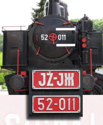
Compound saturated-steam tank engine JŽ 52-011 (former kkStB 178.204) with the axle arrangement 0-8-0T (Dt n2v), now plinthed as a monument in Laško, was built in 1918 under the serial number 7314 by locomotive works Krauss&Comp. in Linz. She shunted in Celje, worked trains to Velenje and later ended her service in the Metalna factory in Maribor. Locomotives of the JŽ 52 class were very popular freight locomotives. They are characterised by Gölsdorf's modification of Heusinger valve gear.
