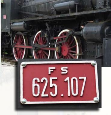
Simple-expansion superheated Italian State Railways steam locomotive FS 625.107 with the axle arrangement 2-6-0 (1'C h2), now plinthed as a monument in Šmartno ob Paki, came to Slovenia within the museum exchange. She was built in 1914 under the serial number 490 by the locomotive works Constr. Meccaniche di Saronno in Italy. In the World War II locomotives of this type worked trains in Istria and Gorica region. Because of their elegant appearance and smooth running they were nicknamed »lady«.
