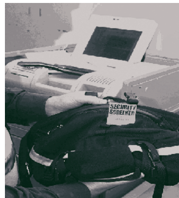
Usage of hand-held ETD equipment that searches for traces of explosive residue on checked-in baggage (Photo DITRDLG)
