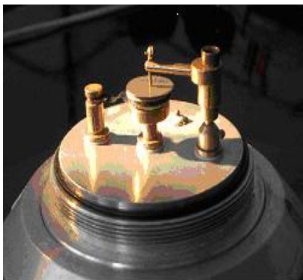
Fig. 4. The inside section of the EasyTest Cell .
