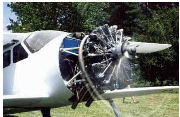
↓ The engine started with only one glitch, a small fuel flow totalizer leak. Although this particular engine had not been run for two years, it started quickly and ran smoothly. Sam Thompson of Tulsa Aircraft Engines provided this slightly used 985 for testing purposes. Because it has already been broken in with 600 hours, we can concentrate on testing Lionheart, rather than the engine.
