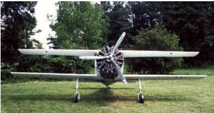
↑ Much of the morning was spent trying to get Lionheart out of the "high bay" area. The ailerons, flaps and wingtips had to be removed in order to get out of our widest door. The cowling is also removed for engine access, in case a few leaks need to be fixed.
