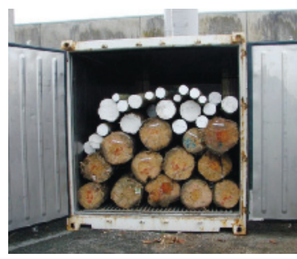
Fumigation trials such as this one, testing efficacy on infested logs, will provide more data on alternative treatments to methyl bromide.
