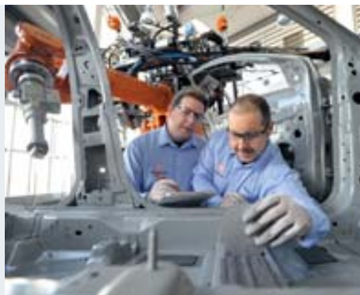
Application engineers Mario Werner (left) and Harald Nees have just applied a sound-damping coating to a car body with the aid of a robot-assisted application system. Now, Harald Nees is checking the layer thickness.
