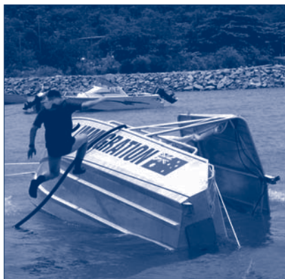
Buoyancy and stability testing of the Malu Sara 's sister vessel by ATSB marine investigators (Photo DOTARS)
