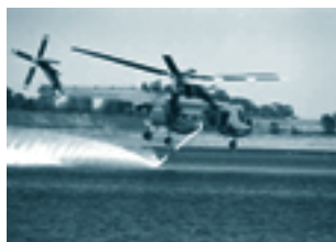
Above: ‘Elvis’ and other Erickson Air-Crane helitankers funded under this programme became a familiar sight to people affected by the January 2003 bushfires. The helitankers can drop up to nine tonnes of water at a time and refill from nearby dams or lakes. (Photo DOTARS)
