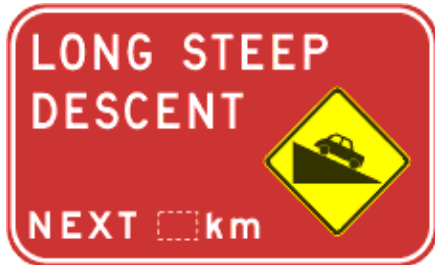
Figure 4: Long Steep Descent sign
