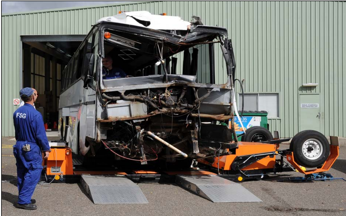
Photograph 7: Coach being placed on RTA VIT
