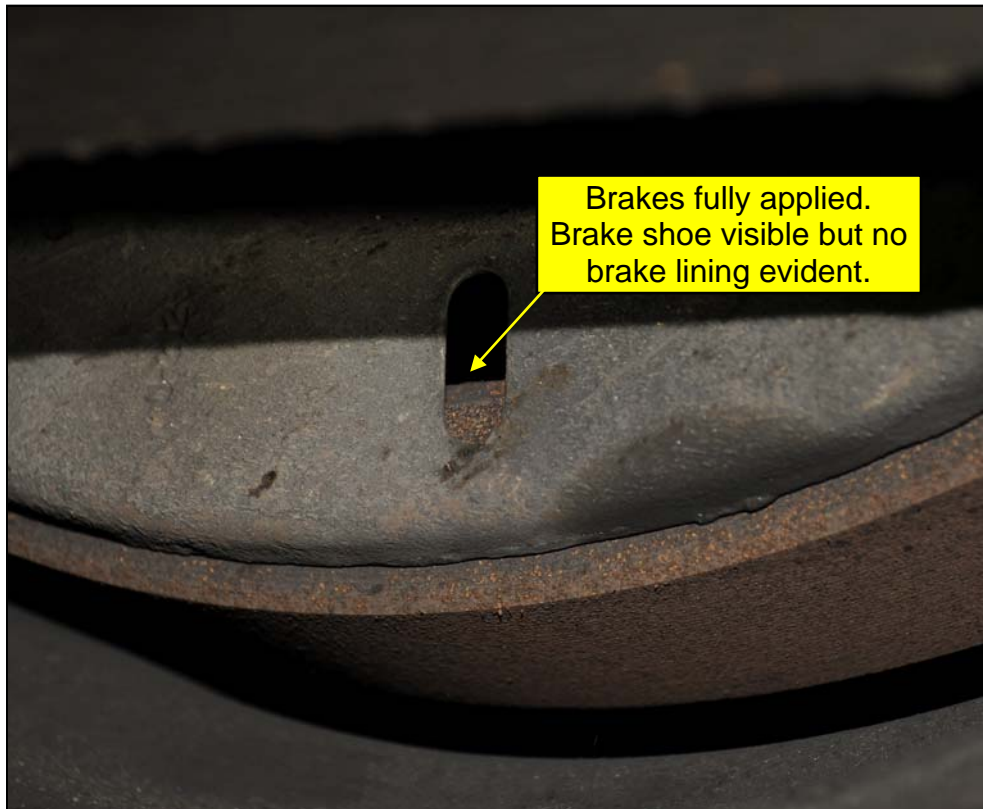
Photograph 8: View of inspection hole of rear brakes in the applied position
