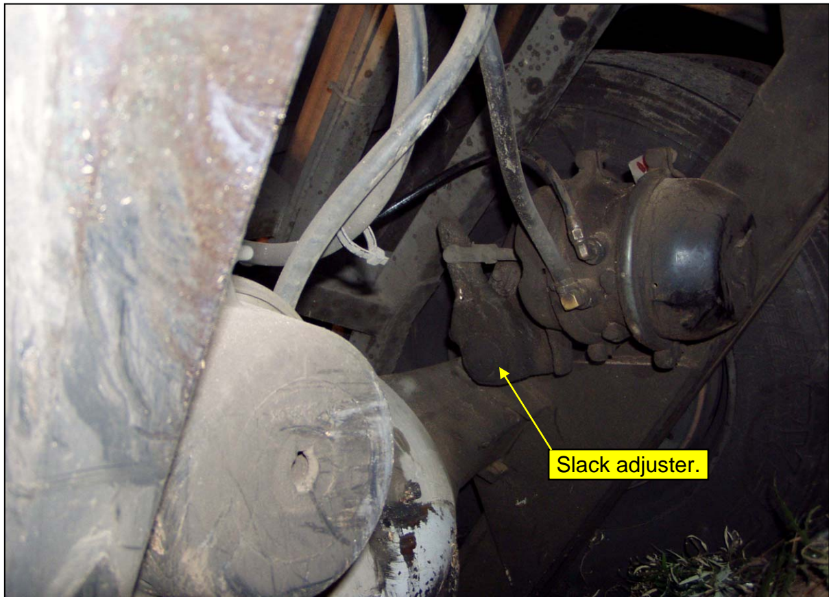
Photograph 11: Condition of brake slack adjuster
