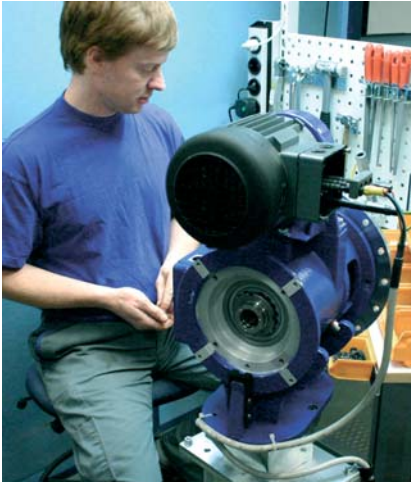
Assembling an MEK-2300 rotating consistency transmitter.
