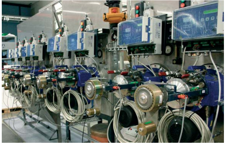
Before shipping, each consistency transmitter undergoes final testing according to ISO 9001 standard.
