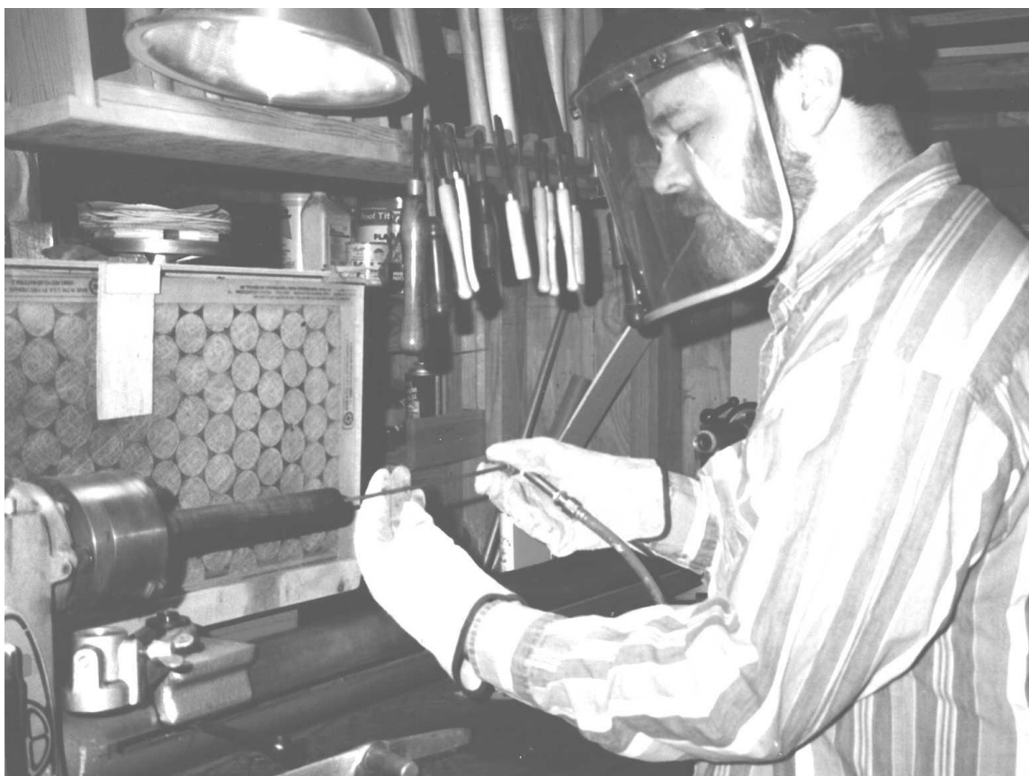
Gun-drilling a bore at "Liestman's House o' Pipes" (some safety equipment removed for photographic purposes) - 100 PSI air pressure going down a 1/32" hole - Now THAT is Livin' !
